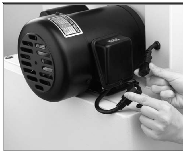
Figure 16. Plugging motor to switch.
